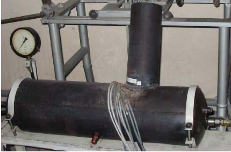
Masurari tensometriche la vase sub presiune
